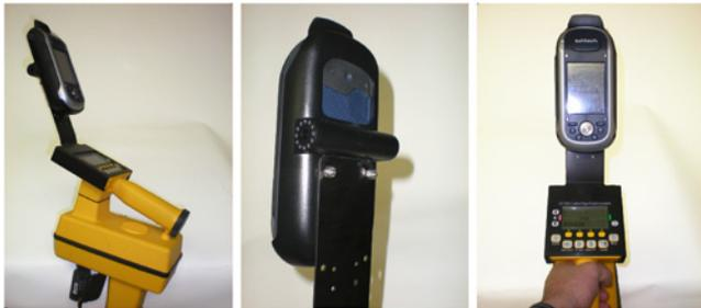
1. Make sure you have configured your Bluetooth adapter to 4800 baud. A Roving BluePort-XP is used. The Bluetooth Pass Code is “1234” on this device.
